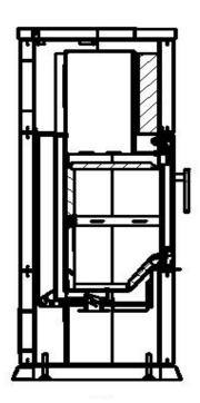
Each smoke baffle plate is removed separately. Both smoke baffle plates are removed by lifting up at one side after which they may come clear at the other side and be taken down into the combustion chamber and out of the door. Similarly, they are put into place by leading them up slanting-wise at one side, and then at the other side, and they are then put into place in the middle.
